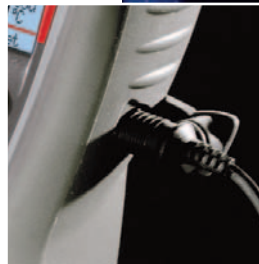
Temperature probe socket and interface for additional sensors
