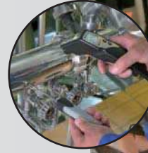
Temperature measurement with external probe
