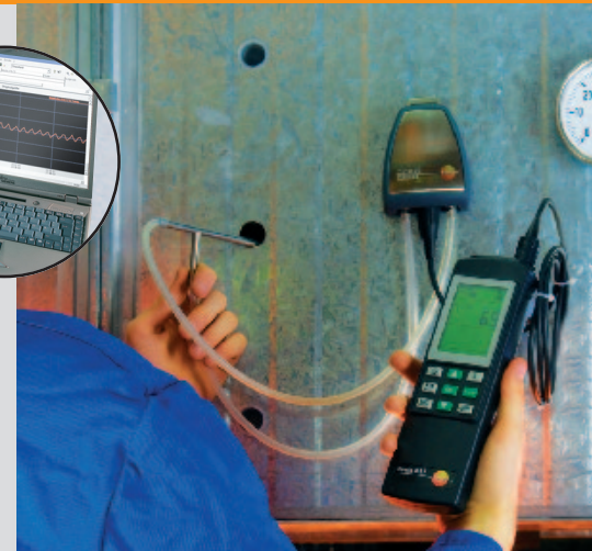
Pitot tube measurement with external 100 Pa probe
